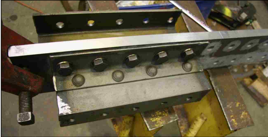
Figure 3.36 Guardrail Bolted to Middle Plate
