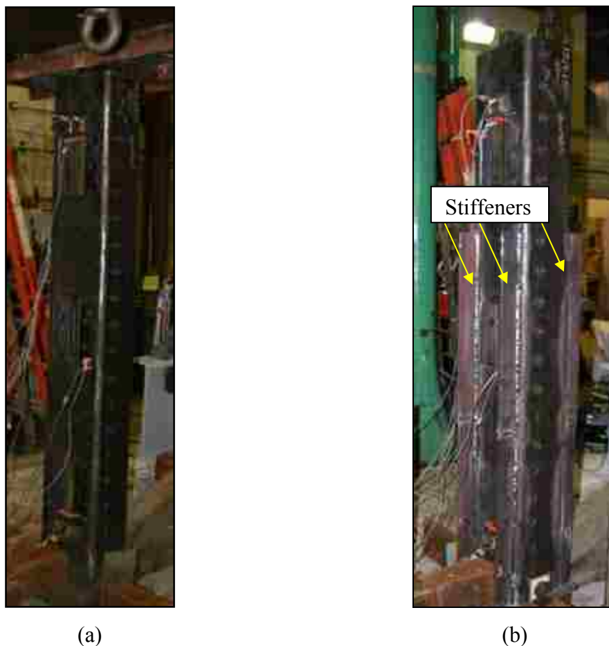
Figure 4.51 Specimen 11R with HSS Reinforcement (a) Prior to Reinforcement (b) After Reinforcement
