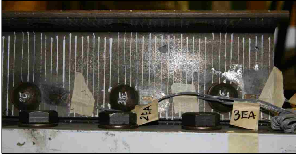
Figure 3.40 Strain Gauge Placement on East Angle
