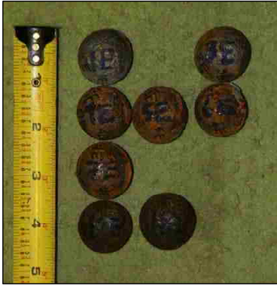
Figure 4.60 East Guardrail Fractured Rivets - Specimen 11R
