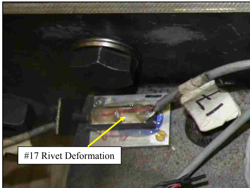
Figure 3.37 Attachment to Guardrail to Measure Rivet Deformation
