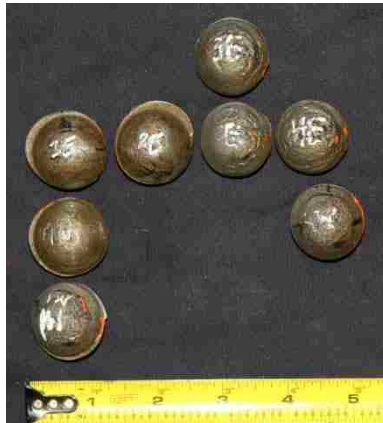
(a) All Fractured Rivets
