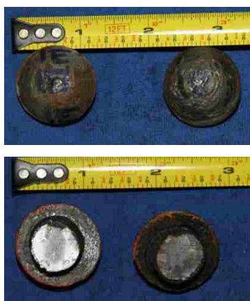
Figure 4.32 Test 2R Fractured Rivets
