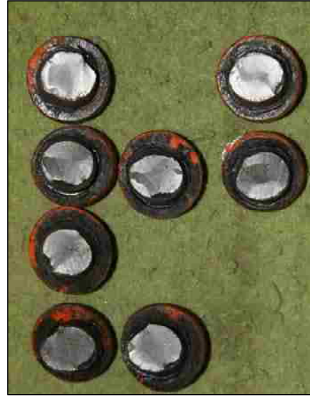
Figure 4.60 East Guardrail Fractured Rivets - Specimen 11R
