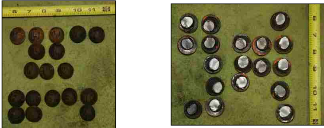
Figure 4.66 West Guardrail Fractured Rivets – Specimen 17R
